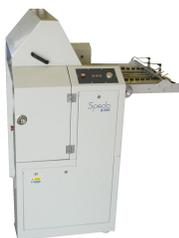
The **SPEDO 6300** in-line, four-plate folder, designed and built to run in system with your Spedo cutter.
